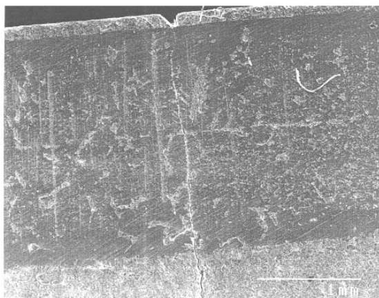
Fig. 3. SEM photo showing a surface layer of TaC and a crack penetrating through a tungsten layer of the target block HIPed using the graphite heater keeping at 1800°C and 2000 \text{kgf/cm}^2 for 3 h.
