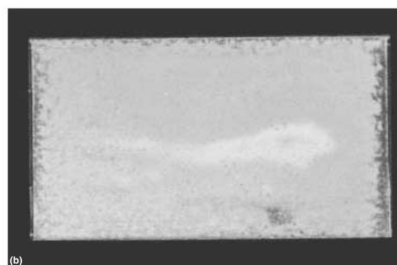
Fig. 10. Ultrasonic echo from the layer near Ta/W interface: (a) block with no hole for thermocouple; (b) first made block with a hole for thermocouple.
